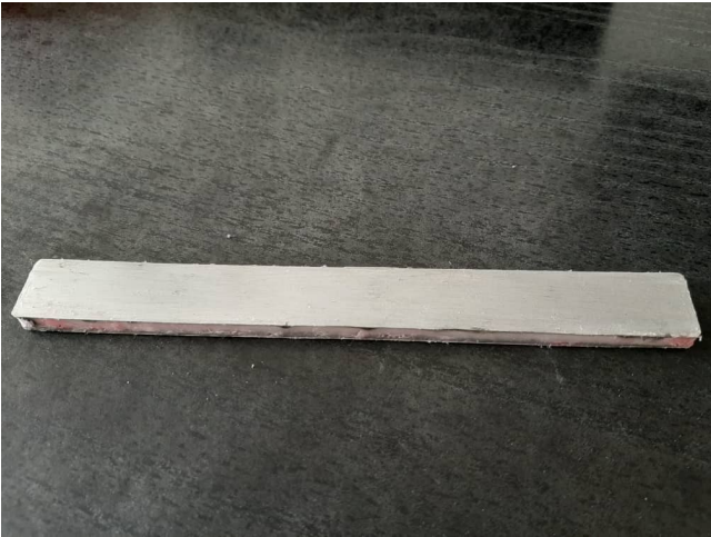
1) Sandwich Beam with 3D Printed Frame Containing MRF (SB-Framed)
