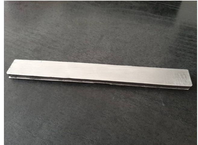
2) Fully 3D Printed Core MRF Layer embedded in Sandwich Beam (SB-Full)
