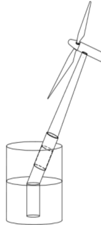
ULS: Failure through plastic hinge of the pile (pile yield failure)
